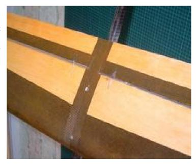
steering wire. This can be made of 1 mm steel. After setting the servo for neutral flying connect the cable to the servo and glue the servo in with epoxy. Then put the aileron horn over the steering wire. Then put some epoxy on the horn and slide it into the slot pulling at the same time the aileron up until it stand neutral. Then let the epoxy cure. A piece of tesa can be taped on the aileron to cover the gap.
